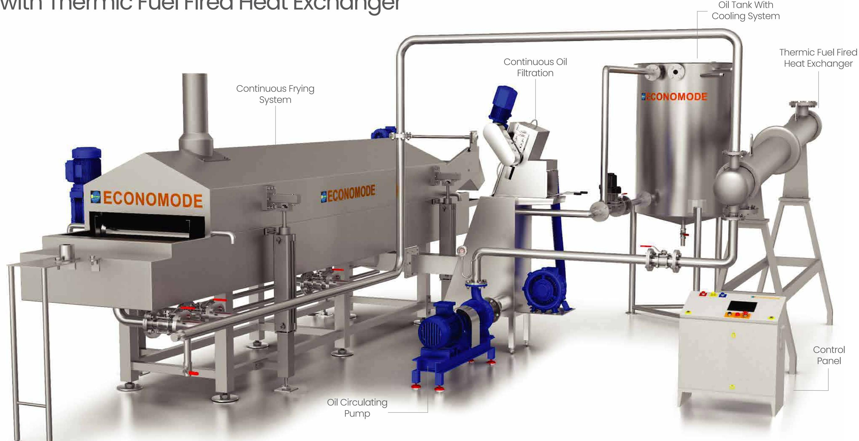
Available in 300/500/1000 Kg per Hour Output Available in Fuel option of Gas/Diesel/Wood/Thermic
